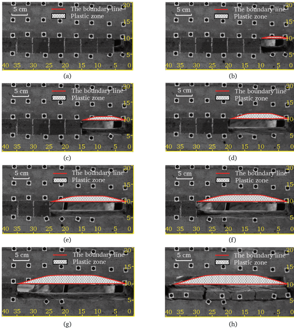
Fig. 19. Comparison of between mechanical model and physical model during the first caving of overburden roof (unit: cm). (a) Advancement distance 5 cm; (b) Advancement distance 10 cm; (c) Advancement distance 15 cm; (d) Advancement distance 20 cm; (e) Advancement distance 25 cm; (f) Advancement distance 30 cm; (g) Advancement distance 35 cm; (h) Advancement distance 40 cm.
