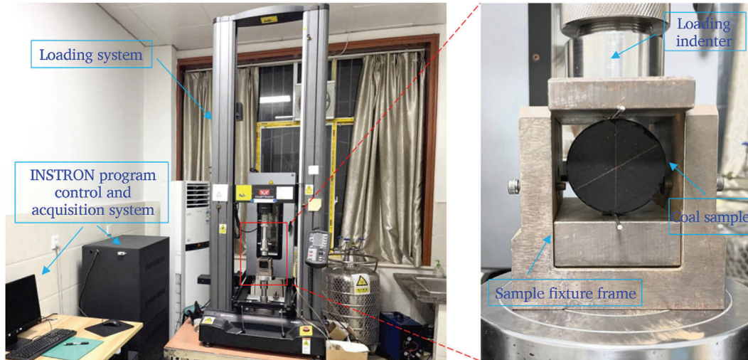
Fig. 3. Schematic diagram of Brazilian splitting loading for coal samples.
