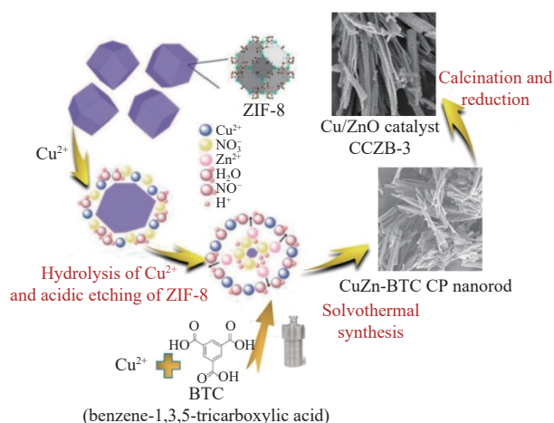
Fig. 1 Schematic diagram of the formation mechanism of CuZn-BTC prepared using ZIF-8 as the sacrificial template [30] (with permission from RSC Publications)
