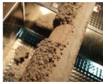
图 2 850 °C 时鼓泡流化床探针上的沉积物 Fig.2 Sediments on probe of the bubbling fluidized bed at 850 °C
