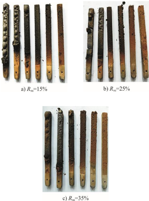
图9 不同细度条件下结渣情况比较 Fig.9 The slagging situations of coal samples with different fineness
