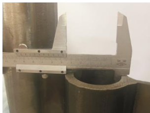
图 16 游标卡尺测量变形 Fig.16 The deformation measurement by caliper
