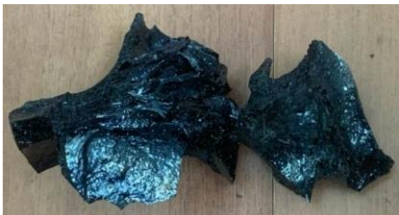
图 3 含铝量高煤种流渣渣块 Fig.3 Slag blockage of high aluminum content coal
