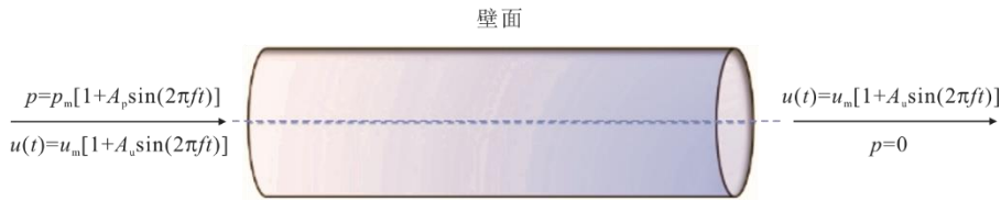
图 2 脉动流仿真边界条件示意 Fig.2 Schematic of boundary condition of pulsating flow
