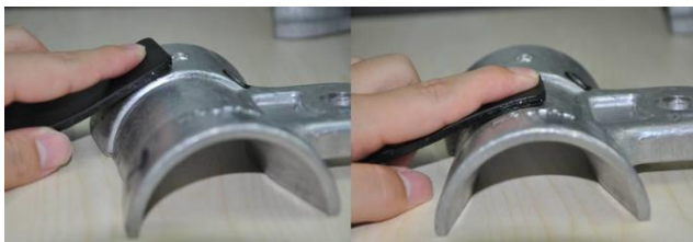
图 12 使用柔性相控阵超声探头检测线夹 Fig.12 Clamp detection with flexible phased array ultrasonic probe
