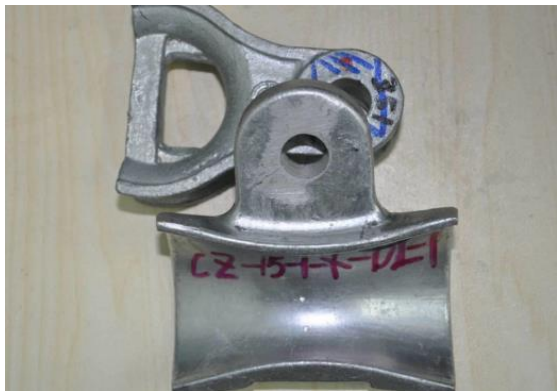
图 11 预埋人工缺陷的线夹 Fig.11 Clamp with artificial defects
