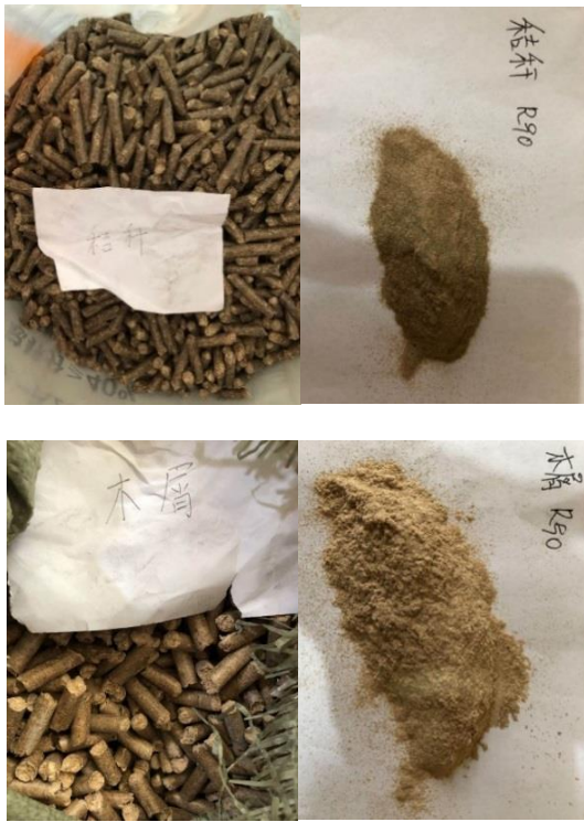
图 5 木屑与秸秆颗粒 R_{90} 磨制效果 Fig.5 Wood chips and straw pellets R_{90} grinding effect
