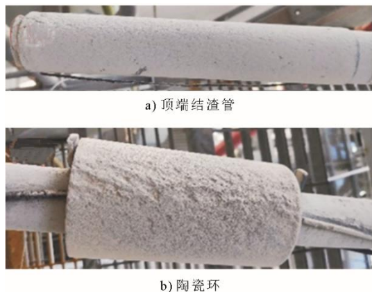
图3 顶端结渣管和陶瓷环沉积样 Fig.3 The depositions on slag tube and ceramic ring
