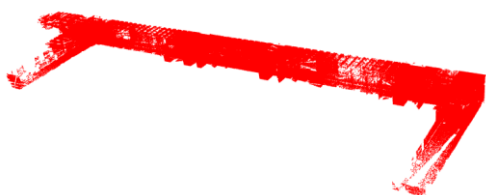
图16 地下管廊完整点云的拼接结果 Fig.16 Complete splicing of multiple point clouds
