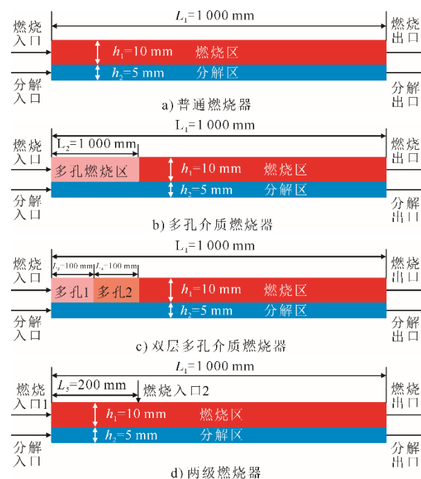
图1 不同燃烧器结构氨燃烧-分解装置计算域 Fig.1 Schematic diagrams of the computational domains for ammonia combustion-decomposition devices with different burner structures
