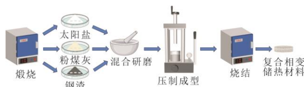
图 2 复合相变储热材料制备流程 Fig.2 The preparation process of composite phase change heat storage materials
