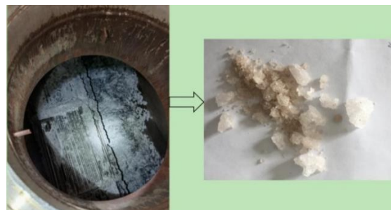
图1 某电厂尿素水解器盘管沉积结晶物( \text{NaCl} ) Fig.1 The crystals ( \text{NaCl} ) deposited on urea hydrolyzer coil of a power plant
