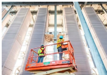
图 4 Heirloom 分层反应器 Fig.4 The layer stack reactor of Heirloom
