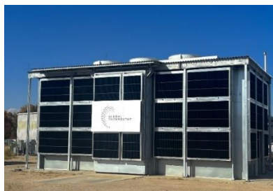
图 2 Global Thermostat 年捕集量千吨级别的示范装置 Fig.2 The demonstration device of Global Thermostat, with an annual CO_2 capture capacity of thousands of tons
