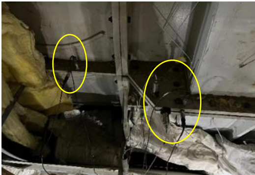
图 3 振动测点位置 Fig.3 Vibration measuring points locations
