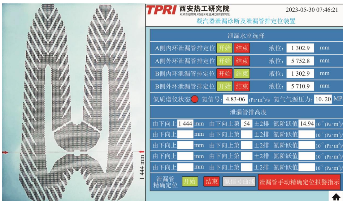
图 7 凝汽器泄漏管排在线定位结果界面 Fig.7 Interface of the result of on-line location of condenser leakage tube row
