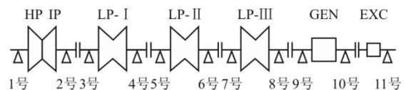
图 3 某 650 MW 核电汽轮发电机组轴系结构示意图 Fig.3 Structure of the shaft system of a 650 MW nuclear power turbo-generator unit
