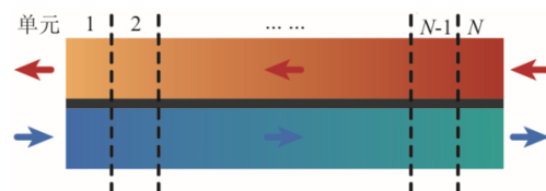
图 4 换热器离散法建模原理 Fig.4 Schematic diagram of principle of discrete method modeling for heat exchangers
