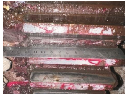
图 14 高黏润滑油脂附着状态下变桨轴承轮齿齿面 Fig.14 Pitch bearing gear tooth surface under high viscosity lubricating grease adhesion state
