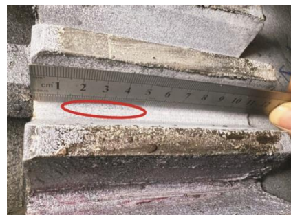
图 15 清理油脂后磁粉检测结果 Fig.15 Testing results of magnetic particle after cleaning oil
