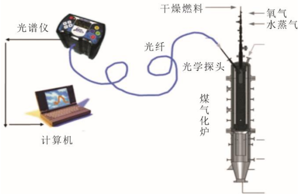
图 3 煤气化炉光谱检测系统结构 Fig.3 The structure of flame emission spectroscopy detection system in coal gasifier
