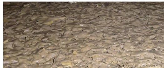
图 3 蒸发冷却器底部沉积的污垢 Fig.3 Fouling deposited at the bottom of the evaporative cooler
