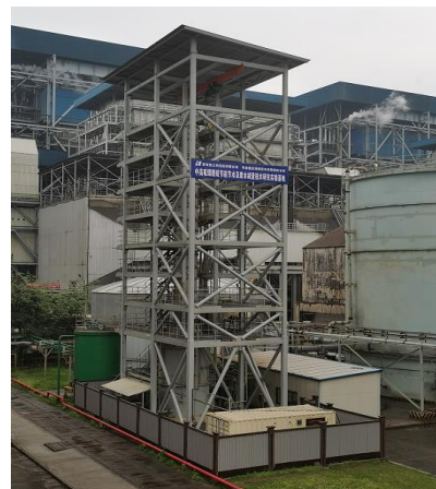
图 1 湿法脱硫大型热态综合试验平台 Fig.1 The large scale thermal test platform for wet flue gas desulfurization
