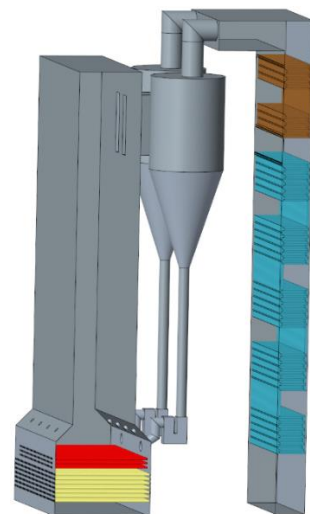
图 1 纯氧燃烧 CFB 锅炉整体布置 Fig.1 The schematic design of the pure oxygen-combustion CFB boiler
