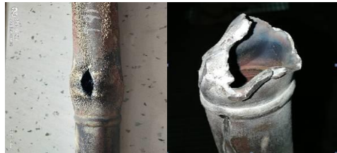
图 16 过热器 TP347 和 T91 对接焊缝后爆口管样 Fig.16 Pipe sample of rear exposure of butt weld of superheater TP347 and T91
