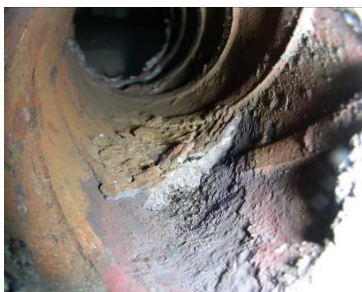
图 7 酸性磷酸盐沉积和腐蚀管样 Fig.7 Acid phosphate deposition and corrosion pipe sample
