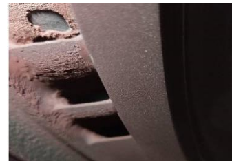
图 5 汽轮机高压调节级表面硅酸盐沉积 Fig.5 Silicate deposition on the surface of high pressure governing stage of steam turbine
