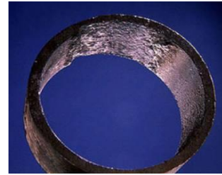
图11 过热水冷壁管段铁氧化物沉积物去除后管样 Fig.11 Removal of iron oxide deposits in superheated water wall
