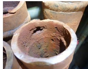
图 17 对接管段内部焊缝凸起爆管管样 Fig.17 Pipe sample of bulged tube blasting for weld of connecting pipe section
