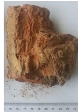
图 8 125 MW 机组锅炉水平烟道堵灰灰块 Fig.8 Ash in horizontal flue of 125 MW boiler
