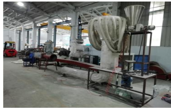
图 1 气固流态化混合分配冷态试验装置 Fig.1 The fluidized gas-solid mixing distribution cold-state device
