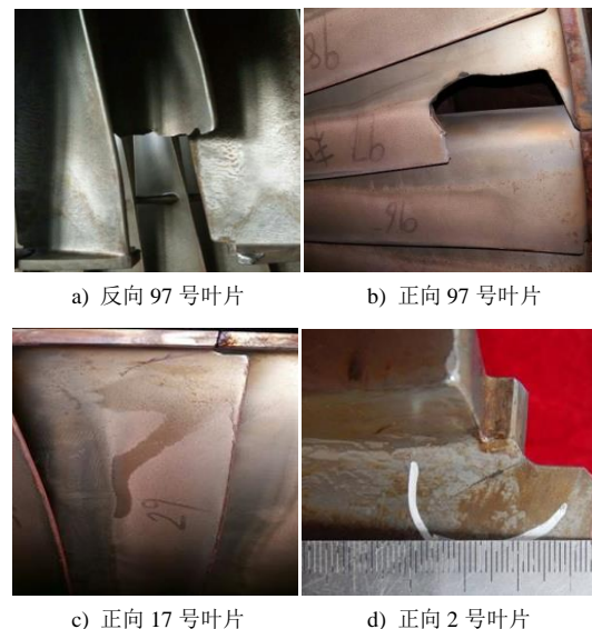
图 1 某汽轮机叶片型线优化前故障情况 Fig.1 Failure situation of a steam turbine blade before optimization
