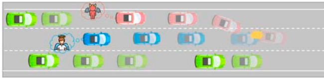
Fig. 6. Adversarial behavior of the environment agent. The blue car represents the ego vehicle driving normally, and the red car represents the environment agent with adversarial behavior.
