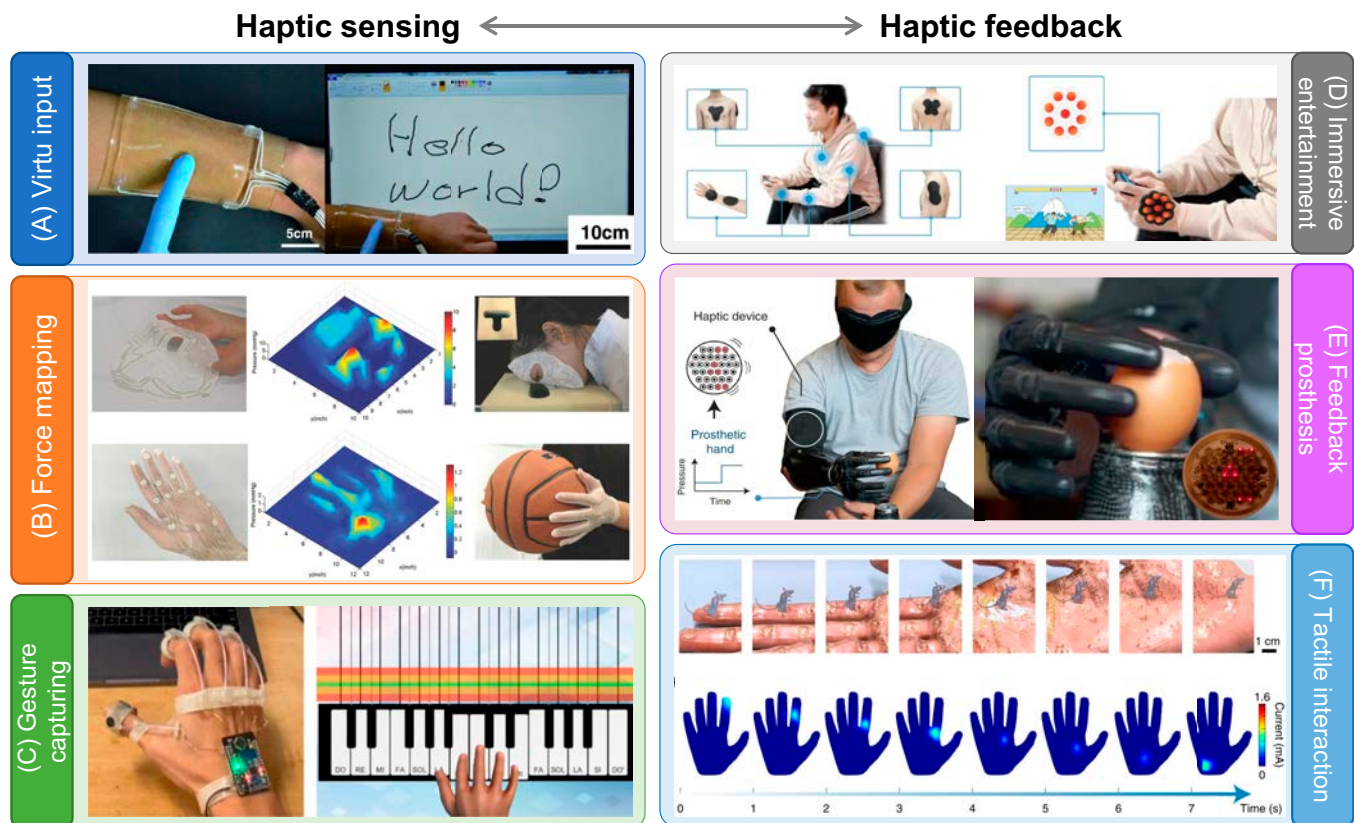
Fig. 16. VR applications of haptic sensors and feedback devices. (A to E) Application examples of haptic sensors in virtual input (A), force mapping (B), and gesture capturing (C), as well as haptic feedbacks in immersive entertainment (D), feedback prosthesis (E), and tactile interaction (F). Reproduced with permission from [7,136,178,179,181,183]. Copyright, the American Association for the Advancement of Science, John Wiley and Sons, and Springer Nature.
