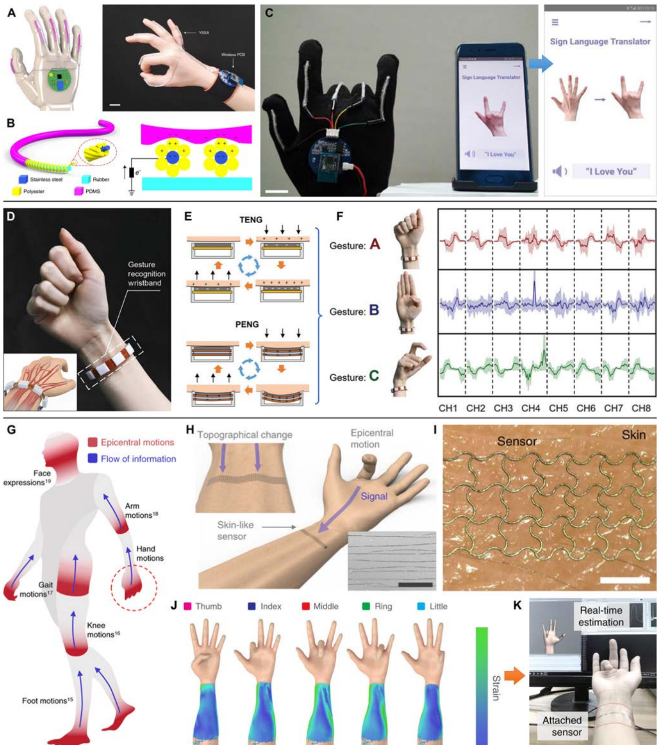
Fig. 5. Tactile sensing devices of gesture recognitions for VR applications. (A to C) Schematic illustration of the triboelectric yarn sensor array (A), working principle (B), and the wearable sign-to-speech translation system (C). Reproduced with permission from [101]. Copyright 2020, Springer Nature. (D to F) Photograph of the gesture recognition wristband sensor (D), working principle (E), and gesture data processing (F). Reproduced with permission from [102]. Copyright 2022, John Wiley and Sons. (G to K) Schematic depicting the possible flow of body information with the epicentral sensor (G), illustration of measuring the epicentral motions of fingers (H) with the insert scanning electron microscopy (SEM) image of the cracked sensor (scale bar, 40 \mu m), photograph of the sensor conformably on skin (I), depiction of skin deformations for different finger bending motions (J), and photograph of the system for gesture duplication (K). Reproduced with permission from [104]. Copyright 2020, Springer Nature.
