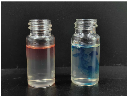
左：苏丹Ⅳ；右：亚甲基蓝。 Left: Sudan IV; Right: Methylene blue. 图 6 染色法鉴定纳米微乳液类型 Fig. 6 Dyeing method to identify emulsion types
