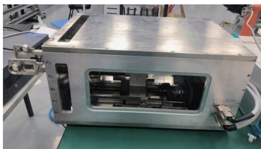
Fig. 7 Double-slit emittance meter
