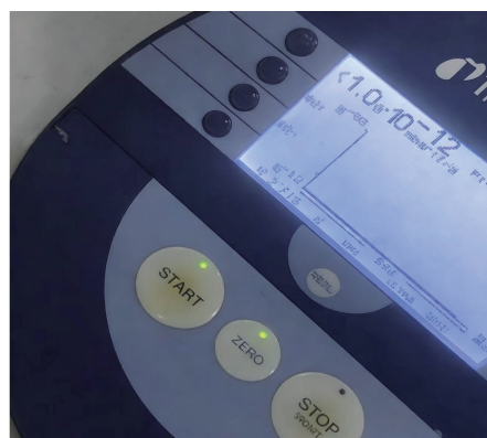
Fig. 10 Leakage rate test
