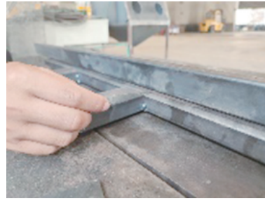
(e)长纵梁中间部位变形检测
