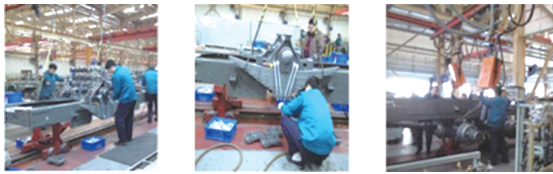
(a)落装平衡轴 (b)安装板簧、U型螺栓 (c)U型螺栓拧紧
