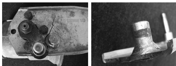
(a)制动阀支架形貌 (b)制动阀支架断口形貌
