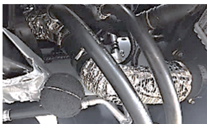
(b)中冷器出气管路近场噪声采集
