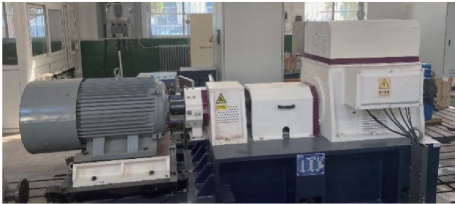
图 14 纯电驱动拖拉机动力系统性能试验台架 Fig. 14 Pure electric drive tractor power system performance test bench
