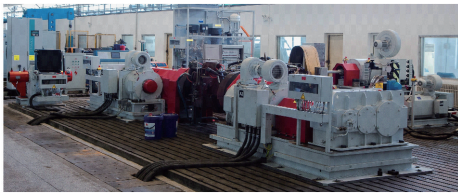
图3 传动试验台架 Fig.3 Transmission test bench
