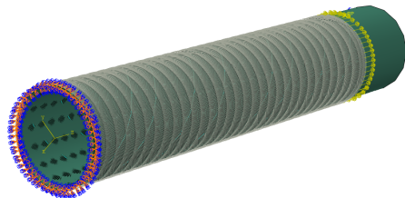
图6 补偿增强层与传感器缠绕成型仿真模型边界设置 Fig.6 Boundary setting of compensation enhancement layer and sensor winding simulation model
