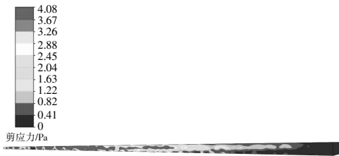
图6 叶片表面流体的剪应力 Fig.6 Shear stress of fluid on blade surface
