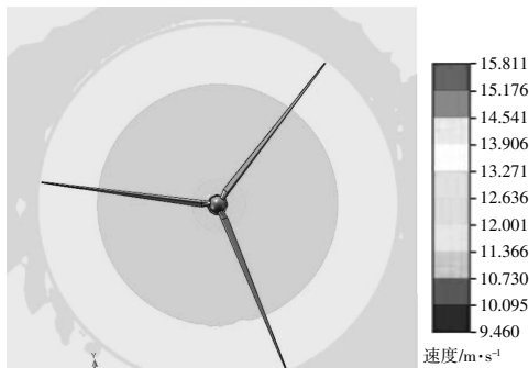
图7 风力机外流场速度分布 Fig.7 Velocity distribution of wind turbine outflow field
