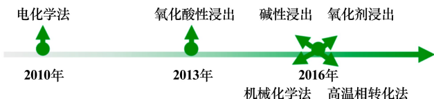
图 3 废旧磷酸铁锂电池选择性浸出回收技术发展路线图 Fig.3 Technology roadmap for recycling of spent lithium iron phosphate batteries by leaching process
