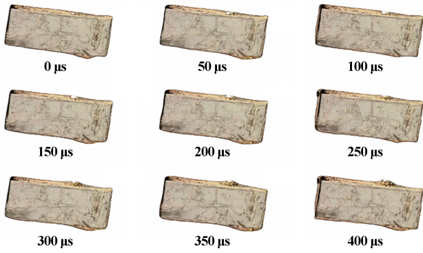
图8 节理宽度 2 cm 条件下单节理岩体爆破裂纹扩展过程 Fig. 8 Blast-induced crack propagation in single-joint rock with joint width of 2 cm
