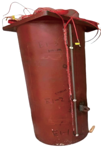
图3 吸力锚及土压传感器布设 Fig. 3 Suction anchor and earth pressure sensor arrangement
