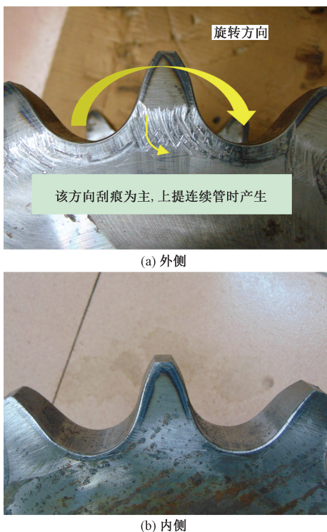
图3 传动链轮 B 端齿侧形貌 Fig. 3 Morphology on the tooth side of the B-end gear of the transmission sprocket
