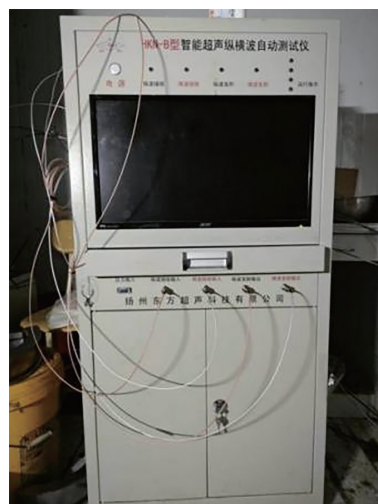
图5 HKN-B 型智能超声纵横波自动测试仪 Fig.5 HKN-B intelligent ultrasonic crosswave automatic tester
