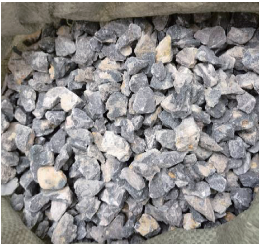
图3 筛分后的5~20 mm再生粗骨料 Fig. 3 Regenerated coarse aggregate of 5~20 mm after screening
