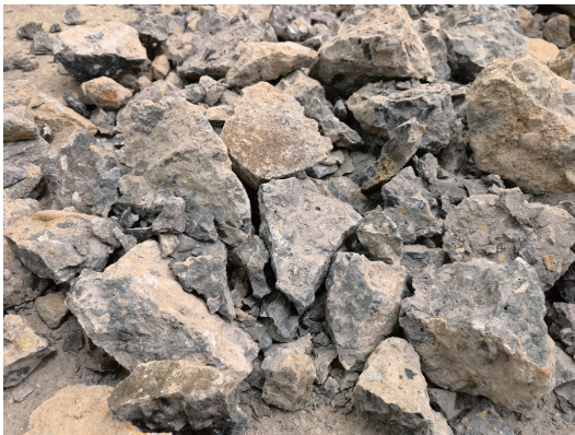
图2 破碎后的再生骨料 Fig. 2 Regenerated aggregate after crushing
