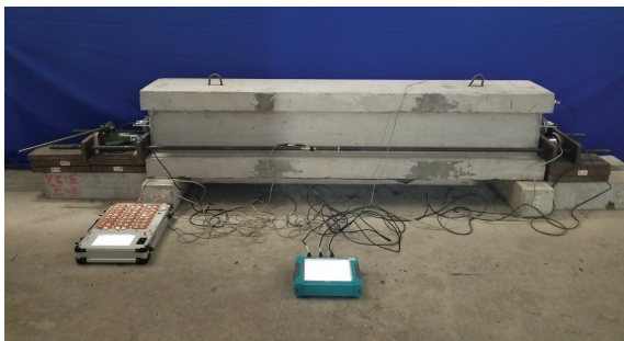
图8 偏心受压试验现场加载示意图 Fig. 8 Field loading diagram of eccentric compression test
