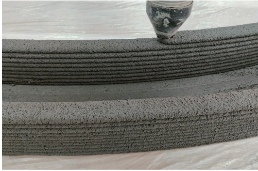
图 3 3D 打印混凝土条带效果 Fig. 3 3D printed concrete strip effect
