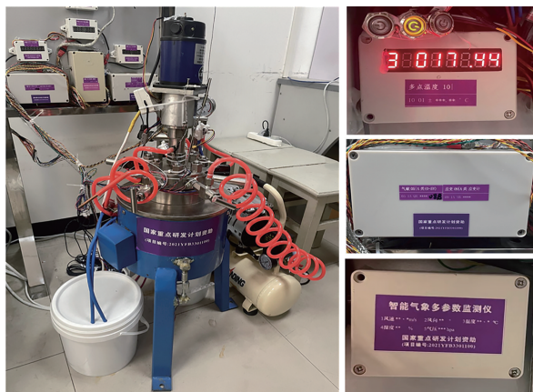
图4 反应釜工作场景和部分传感器 Fig. 4 Working scene and some of the sensors of reactor
